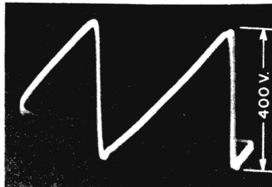
FIG. 39. WAVEFORM - OUTPUT OF HORIZONTAL OSCILLATOR - UPPER HALF (JUNCTION OF R-46 AND C-53 AND B-)
